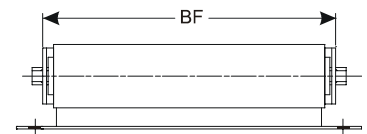
C1285 Required with int. drive 2.56" dia. x .180" roller with power service bearings and 1 1/16" hex axle
